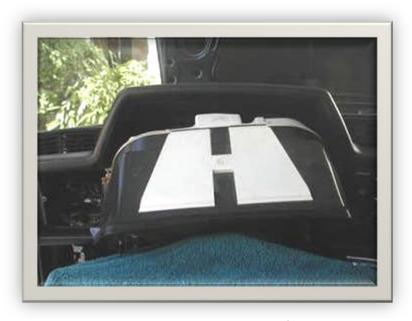
Place a thick towel or other padded covering over the top of the steering column. Gently pull the instrument cluster out to lay face down on the top of the steering column.
