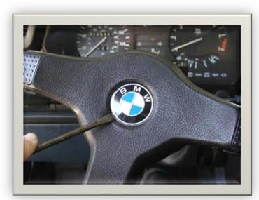
Using a bladed screwdriver
