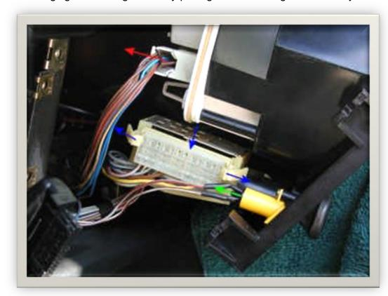
Remove the head light switch light bulb by pulling the bulb straight out of the yellow holder (green arrow).
