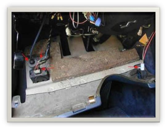
Remove the connectors and vacuum hose from the knee panel mounted equipment. Note where they came from...or take pictures beforehand.
