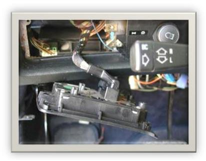
Carefully pull the module out so that the connector to the cable bundle at the back of the check panel module is accessible. Carefully disconnect the wire bundle connector and set the check panel module aside in a safe place.
