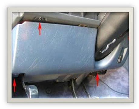
Remove 4 screws to remove the knee panel.
