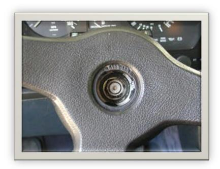
Using a 22mm socket with a 3 inch or more extension, remove the steering wheel nut. Before removing the steering wheel, note the V shaped mark etched on the spindle, and the line etched on the steering wheel adjacent to the hole. These are the reference points for properly installing the steering wheel. Remove the nut and the steering wheel from the spindle.
