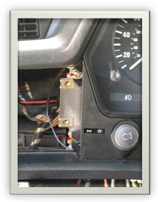
Remove the 2 left side instrument cluster mounting screws.
