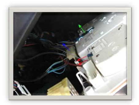
Disconnect the odometer wires (red arrows), the main SI board bundle connector (blue arrow), and the Gas/Temp gauge bundle connectors (green arrow). Connectors should be disconnected in the direction of the arrows. Be careful to pull the connector straight out and to not break the connector.
