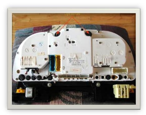
Lay the instrument cluster face down on a soft, well padded surface. A throw pillow works nicely. If you are changing the instrument cluster light bulbs, this is the time to do it.
