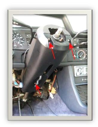
Loosen the steering column lever to gain access to and remove 3 screws holding the bottom steering column cover.
