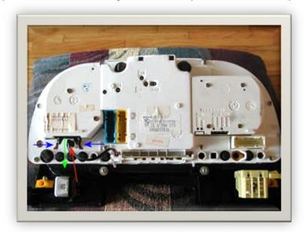
If you will be removing the tachometer for some reason, you will need to: Remove the real-time mileage gauge wire (red arrow)
