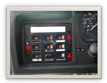
Remove 3 screws holding the check panel module in place.
