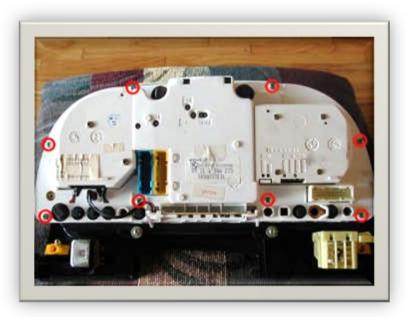
Remove the 8 instrument cluster screws. Gently pull the instrument cluster electronics straight up and out of the body. Set the body and the pillow aside.
