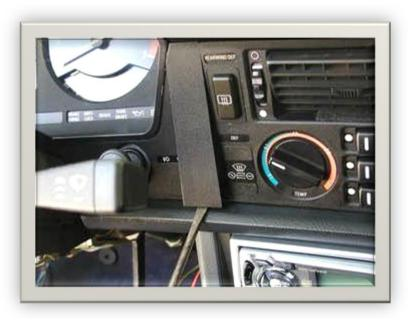
Using a thin bladed screw driver, carefully pry loose the molding to the right of the instrument cluster.
