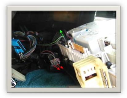
Disconnect the fog light switch wires (red arrows) and the Anti-Lock instrument bulb (green arrow)
