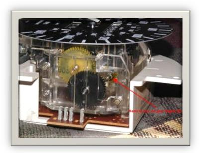
Inspect the gears on the right side of the speedometer. It is advisable to replace the first three gears as they will all fail.
