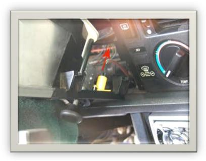
Remove the fog light switch light bulb by pulling the bulb straight out of the yellow holder.
