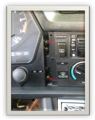
Remove the 2 right side instrument cluster mounting screws.
