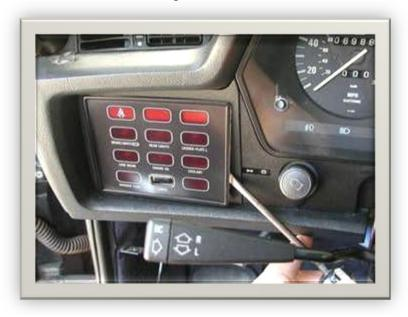
Using a thin bladed screw driver, carefully pry the bottom of the check panel cover out. The check panel cover is held in place with 2 tabs at the top. Do not try to pry the cover off from the top.
