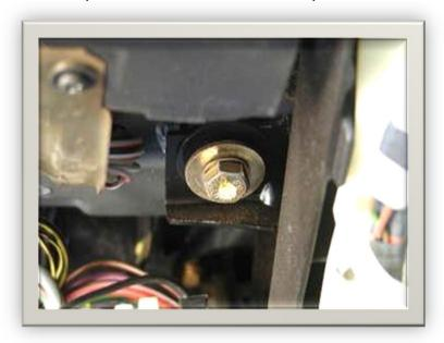
Use a 13mm socket wrench to remove 2 bolts on either side of the steering column. These hold the steering column in place. When removing the second bolt, support the steering column and gently lower it until it rests in place.
